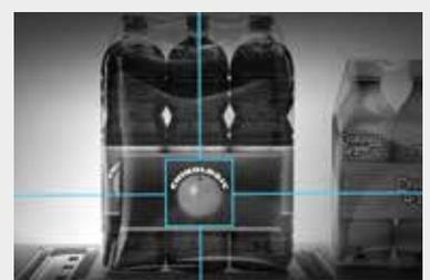
Its capability to manage large databases of patterns allows Pattern Sorting Tool to distinguish among thousands of different items manufactured or travelling on a conveyor. The algorithm delivers robust recognition in any situation: 360° pattern rotations, perspective distortions, different scales and light variations.
