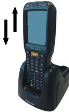
Figure 2 - Mobile Computer Insertion
