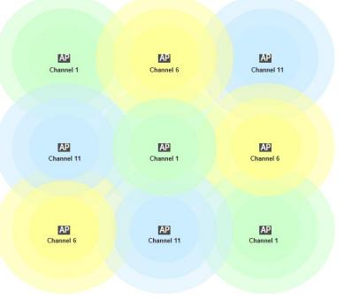
A typical Wi-Fi deployment is a set of overlapping "cells" of coverage.
