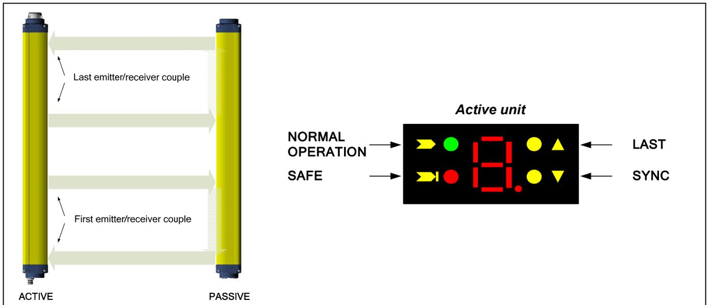
Signals are clearly identified through symbols allowing immediate reading, independent of bars directions. A short description of the signalling LEDs is necessary to avoid misunderstandings. Two yellow LEDs (▲ LAST, ▼ SYNC) on SG-BODY Reflector active unit facilitate the alignment procedure.
