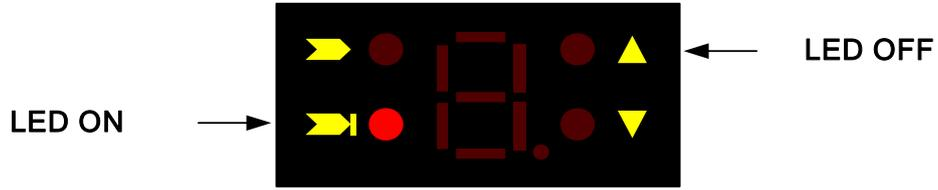
The operator can evaluate the main causes of the system stopping or failure using the 7-segment display and LEDs used to visualise the functions.
