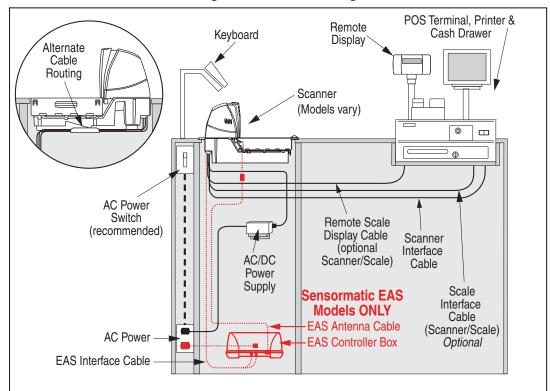
Figure 2-13. Cable Routing
