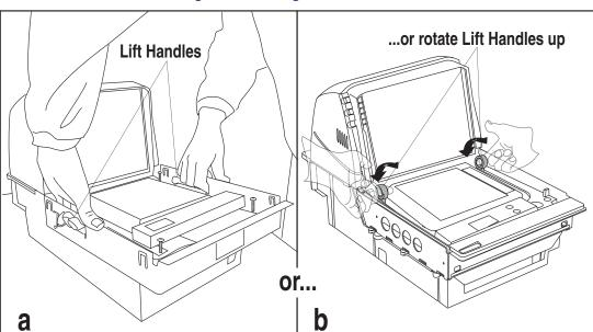
Figure 2-25. Using the Lift Handles
