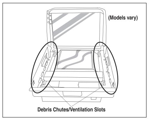
Figure 2-3. Debris Chutes & Ventilation Slots
