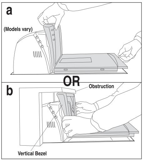
3. Depending upon the model type, the method used to lift the unit will vary. For the first model type, hook the fingers of both hands into the lift handles located along the insides of the scanner walls, just above the debris chutes as shown in a. Other models contain lift handles that must be rotated up into position for use as shown in b. DO NOT attempt to lift the unit using the plastic edges, scale frame, or any features other than the lift handles.
