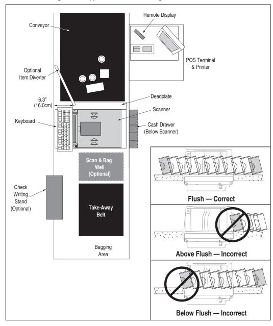
Figure 2-5. Typical Checkstand Design & Cutout Location
