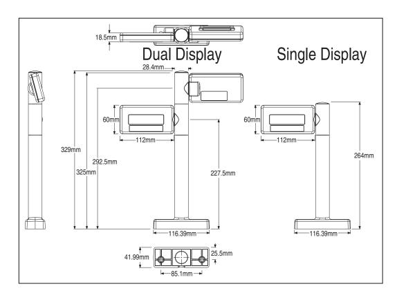
Figure 2-16. Model 8300RD Physical Measurements
