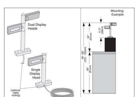
Figure 2-17. Model 8300RD Remote Scale Display Mounting
