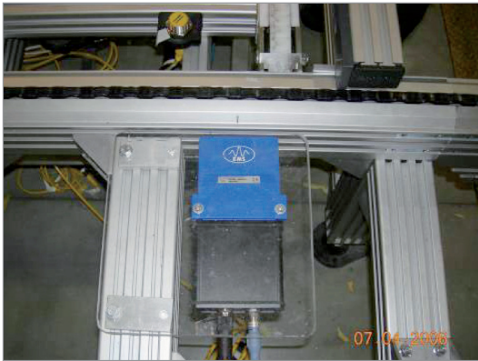
.Escort Memory Systems COBALT™ RFID Controller/Antenna in a conveyor section
