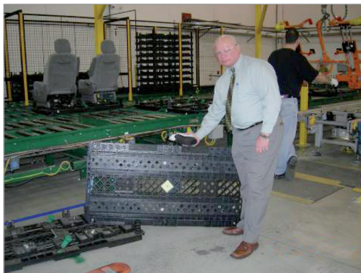
.Shipping Pallet with an Escort Memory Systems durable RFID tag
